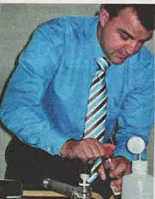
Tiny particles of dust, sand, metal, glass, sludge and rust that are invisible to the human eye are just some of the money sapping foreign bodies found in diesel samples tested by Niko Verhaegen, development manager for filtration experts Donaldson.
